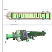
Designs for an AES type heat exchanger.
